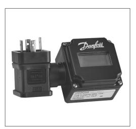
A microprocessor controlled plug-in display that can be universally applied to all MBS, AKS and MBT transmitters with a 4-20 mA output and DIN 43650 plug.
