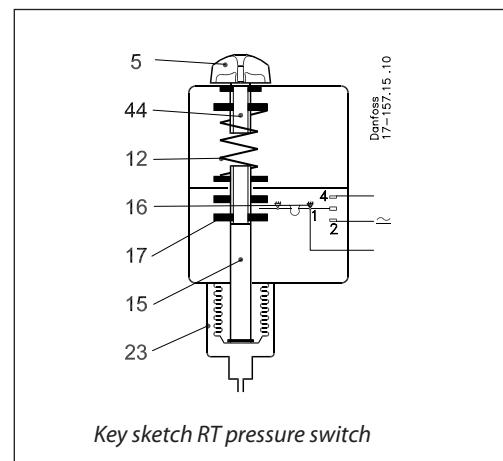
An RT-E differential pressure switch contains single-pole changeover switch that makes or breaks depending on pressure differential between two counteracting bellows elements (LP and HP).
